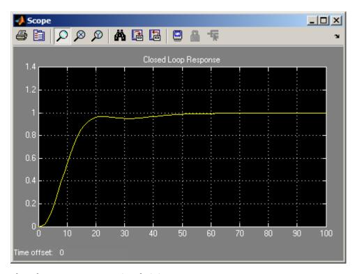
**Closed-Loop Response Using fminimax**
